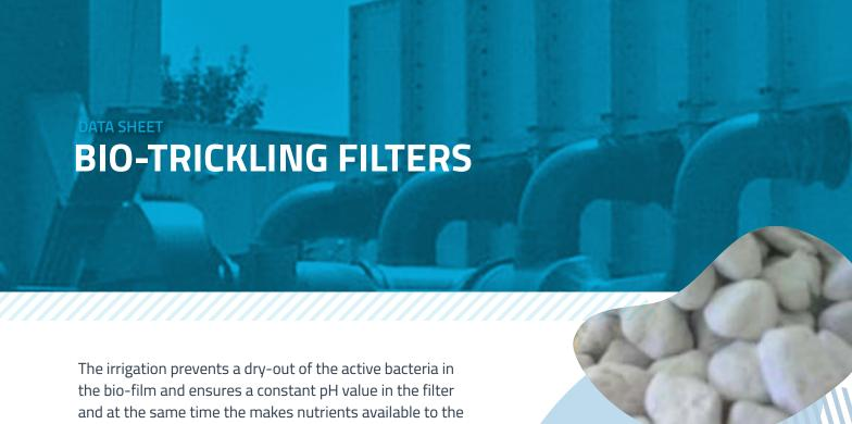
The irrigation prevents a dry-out of the active bacteria in the bio-film and ensures a constant pH value in the filter and at the same time the makes nutrients available to the bacteria. The percolating water collected at the filter bottom contains odour components as well as sulphuric acid from the biological oxidation of hydrogen sulphide.
